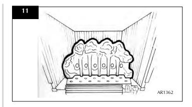
• Place the front coal centrally in the channel at the front of the tray. The relationship between the front coal and the flame baffle is shown, Diagram 12.
